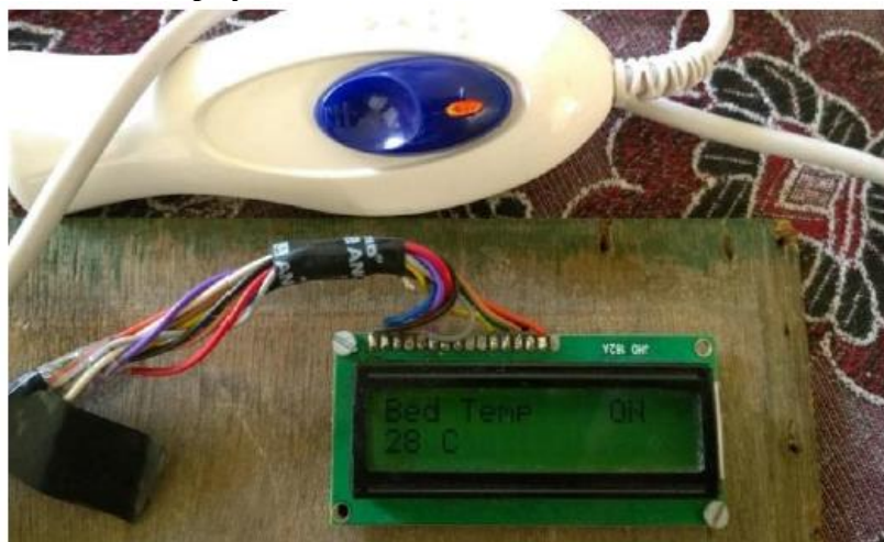
Fig. 3: Bed temperature is detected and is displayed.
