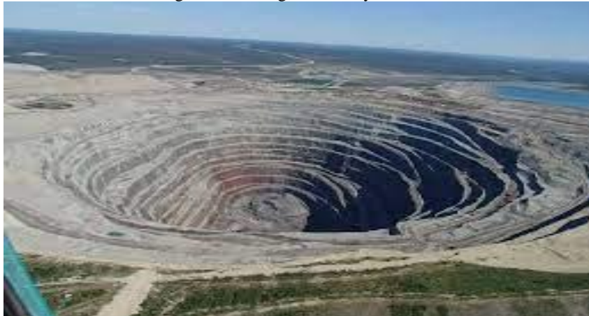
Figure 2: Mining Method by Bench
